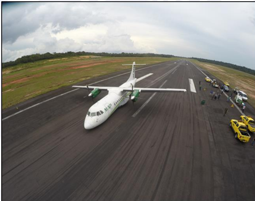
Figure 1 - View of the aircraft after landing at SBEG with the landing gear retracted.
