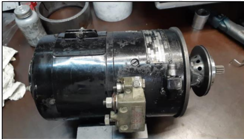
Figure 21 - Overview of the Starter-Generator No. 2.
