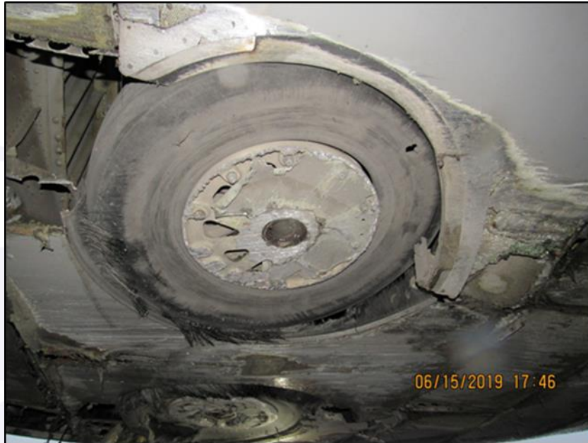
Figure 4 - Damage to the wheels, tires, and landing gear doors.
