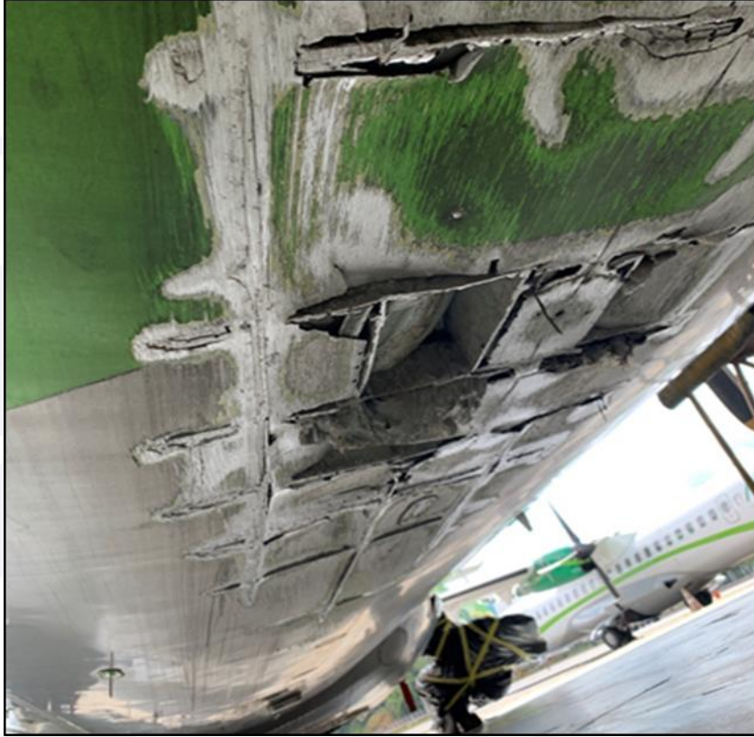
Figure 2 - Damage to the central underside of the fuselage.
